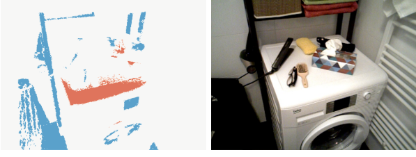
Figure 4. Left: predicted saturation map. Red pixels correspond to the surfels with invalid overexposed colors, blue pixels correspond to the surfels with invalid underexposed colors. Right: color image of the scene.
