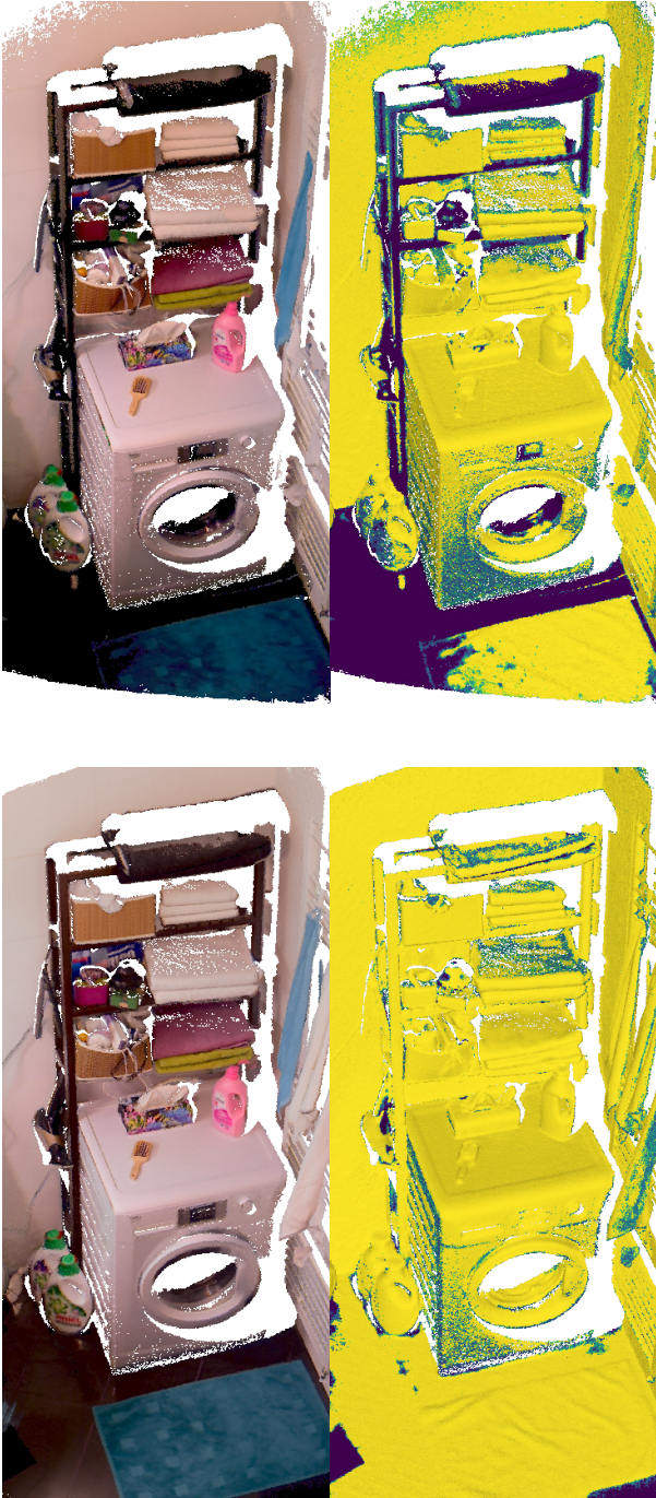
Figure 7. HDR reconstructions obtained using our system, without (top row) and with (bottom row) the custom exposure controller. Left column shows the visual appearance of the reconstruction, right column shows the color confidence of the surfels (color-coded, yellow means confident, dark violet means invalid color).
